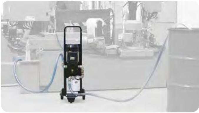
60 l/min filter with head
