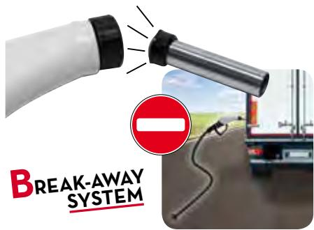
**EN.** Safety is guaranteed by the break-away system. In the event that a vehicle accidentally drives away with the nozzle still in the tank, the spout is designed to detach from the nozzle. This system also allows for a quick repair by merely fitting a new spout onto the nozzle.
