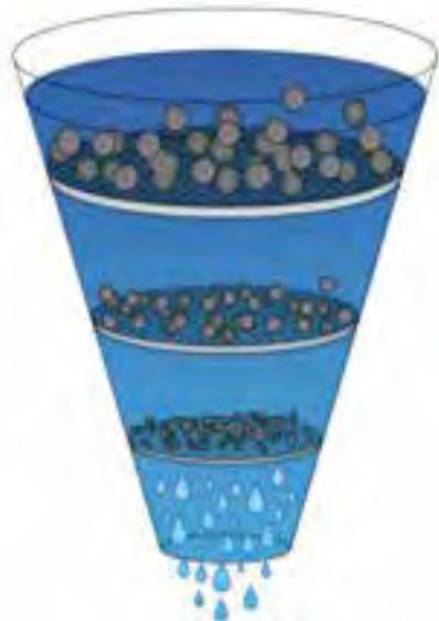
**EN.** High efficiency ( $\beta$  200) mechanical filtration of particulate by means of an incremental filter specifically developed for AdBlue®. We recommend changing the filter cartridge once a year.
