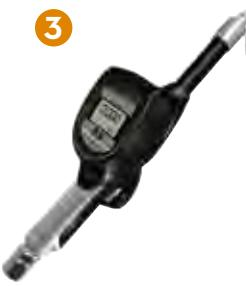
**EASY VIEW** High strength and performance are the core properties of the Easyview nozzle. ENHANCED ERGONOMICS. The nozzle design has been further improved. Easyview is a more practical and more intelligent nozzle. The large size display shows the dispensing data transmitted on a wireless connection (zigbee) from the associated GPV 2.0. This means the nozzle no longer needs an internal flow meter, resulting in a significant weight reduction and less risk of damage.
