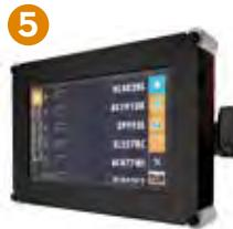
**CONTROL UNIT 2.0** Thanks to static and mobile 2.0 Control Units, you'll have the updated list of pending tasks and their state of completion readily to hand at any time. The touchscreen device allows the operator to scroll through the tasks list, which is constantly updated in real time. Particularly urgent work orders can be highlighted.
